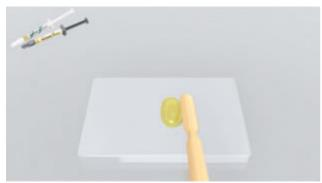
**Variolink N** is mixed on a mixing pad in a 1:1 ratio for 10 seconds (careful spatulation). The working time of the mixed Variolink N is about 3.5 min. at a temperature of 37 °C/99 °F.
