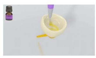
**Monobond N** is applied to the pretreated surfaces with a brush or microbrush and left to react for 60 seconds. Subsequently, it is dried with a vigorous stream of air.
